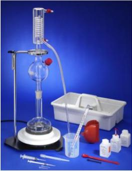
A laboratory setup for volatile acid determination. It features a round-bottom flask on a magnetic stirrer/heater, connected to a vertical glass column (distillation column) with a condenser. A syringe is used for titration. The setup is placed on a white tray. |
