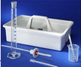
A specialized apparatus for CO2 measurement in still wine. It includes a white tray, a graduated cylinder, and a special measuring vessel (eprouvette) used for shaking the wine to release CO2.                                                                    |
